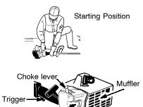
**WARNING:** The trimmer head will turn while starting the engine. Avoid any contact with the muffler. A hot muffler can cause serious burns.
